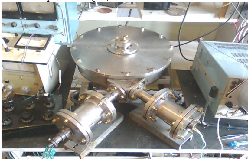
Fig. 1. Photo of a flight mass spectrometer with an axial-symmetric electric field
