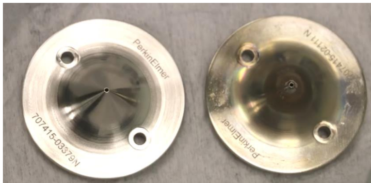
Fig. 10. Conditions of skimmer and sampler after analysis of 25-30 blood samples with (a) addition of 2% oxygen and (b) failure
