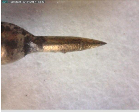
Figure 1. Tungsten needle wetted by Au + Ge alloy
