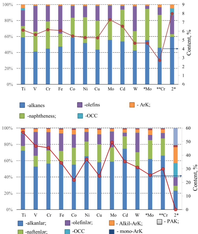
Figure 16. Distribution of group hydrocarbons in fractions I and II oxycracking depending on the nature of modifiers (%).
