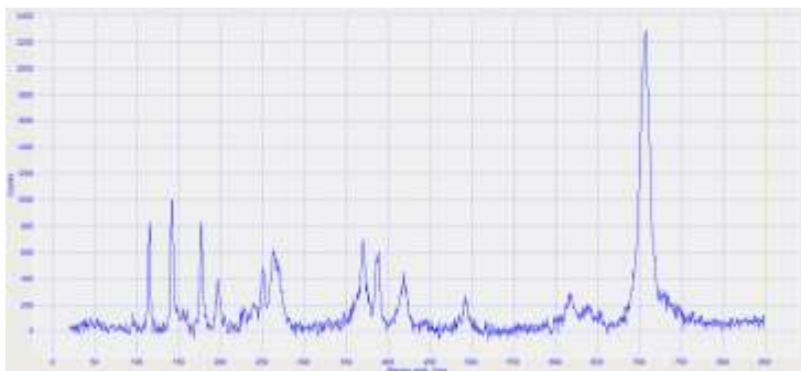
Figure 18. Raman spectroscopy of electrochemically deposited thin Mo-S samples (thermally processed sample). Electrolyte (M):1 \text{Na}_2\text{MoO}_4 \cdot 2\text{H}_2\text{O} + 0.1 \text{Na}_2\text{SO}_3 . Thermal processing – 623 K.
