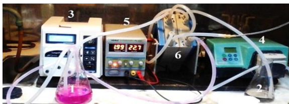
Figure 12. Electro dialysis device (a) 1 – alkaline receiver, 2 – acid receiver, 3 and 4 – rotometer, 5 – voltmeter/ammeter, 6 – PC Cell 64004 electro dialyzer
