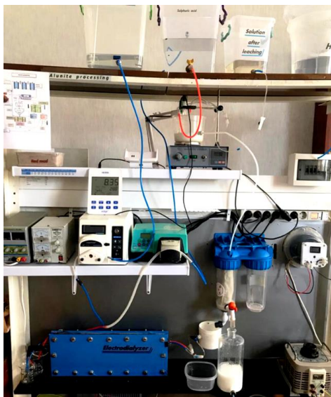
Figure 14. Laboratory mobile pilot plant of the proposed alunite ore processing technology
