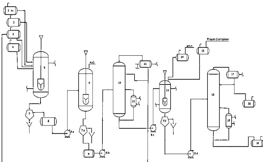
1-H<sub>2</sub>O; 2-cycloolefin; 3-HBr(HCl); 4-oxidizer; 14-amine; 15- containers for propanol-alkali solution, 5-reactor, 6-neutralizer, 7,7a,7b-fluoret, 8- intermediate capacity, 8a,8b,8c,8d-pumps, 9 - capacity for hydroxyhalides, 10,16- rectification column, 17, 18- capacity 12,19 - heater 13- main reactor, 20- capacity for product
