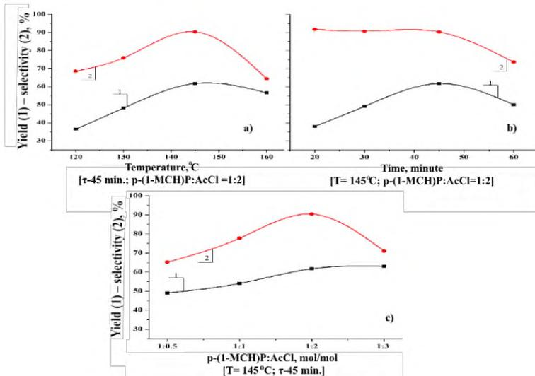
**Fig. 1. The results of acylation reactions of *para*-(1-methylcyclohexyl)phenol with acetyl chloride in the presence of ZnCl<sub>2</sub> catalyst**
