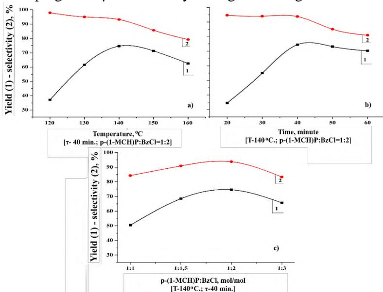
**Fig. 4.** The results of acylation reactions of *para*-(1-methylcyclohexyl)phenol with benzoyl chloride in the presence of dispersion ZnCl<sub>2</sub> impregnated  $\gamma$ -Al<sub>2</sub>O<sub>3</sub> catalyst
