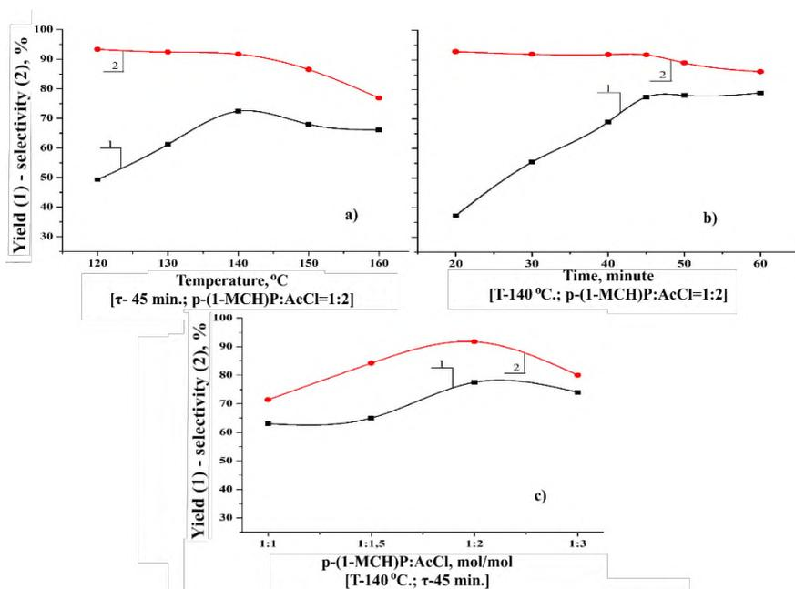
**Fig. 2. The results of acylation reactions of *para*-(1-methylcyclohexyl)phenol with acetyl chloride in the presence of  $ZnCl_2$  impregnated  $\gamma-Al_2O_3$  catalyst**
