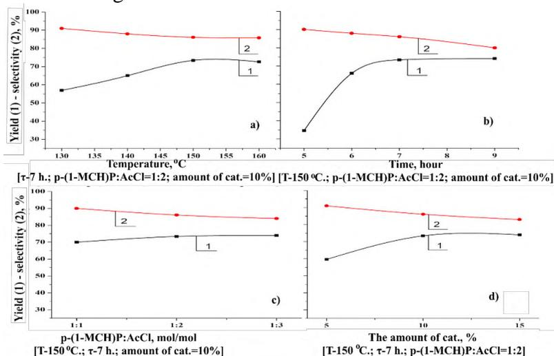
**Fig. 3.** The results of acylation reactions of *para*-(1-methylcyclohexyl)phenol with acetyl chloride in the presence of KU-23 catalyst
