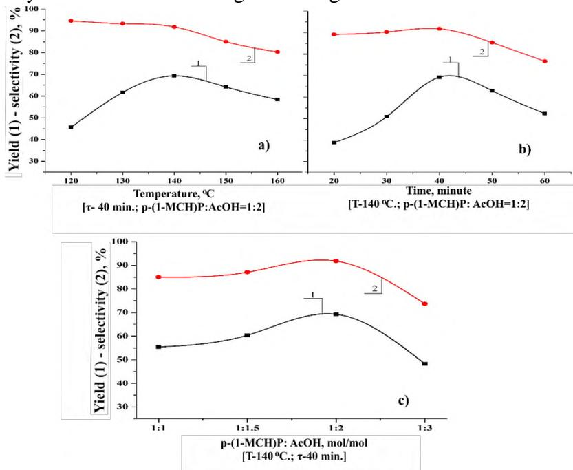
**Fig. 5** The results of acylation reactions of *para*-(1-methylcyclohexyl)phenol with acetic acid in the presence of ZnCl<sub>2</sub> impregnated  $\gamma$ -Al<sub>2</sub>O<sub>3</sub> catalyst
