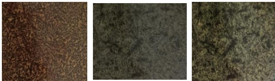
Figure 4. Coatings obtained on the surface of marble slabs based on MPFR: pigment- \text{Fe}_2\text{O}_3 - (a), \text{FeO} -(b), \text{Cr}_2\text{O}_3 - (c)
