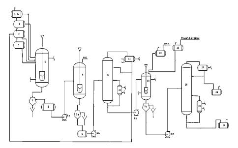
1-H<sub>2</sub>O; 2-cycloolefin; 3-HBr(HCl); 4-oxidizer; 14-amine; 15- containers for propanol-alkali solution, 5-reactor, 6-neutralizator, 7,7a,7b-fluoret, 8- intermediate capacity, 8a,8b,8c,8d-pumps, 9 - capacity for hydroxyhalides, 10,16- rectification column, 17, 18- capacity 12,19 - heater 13- main reactor, 20- capacity for product
