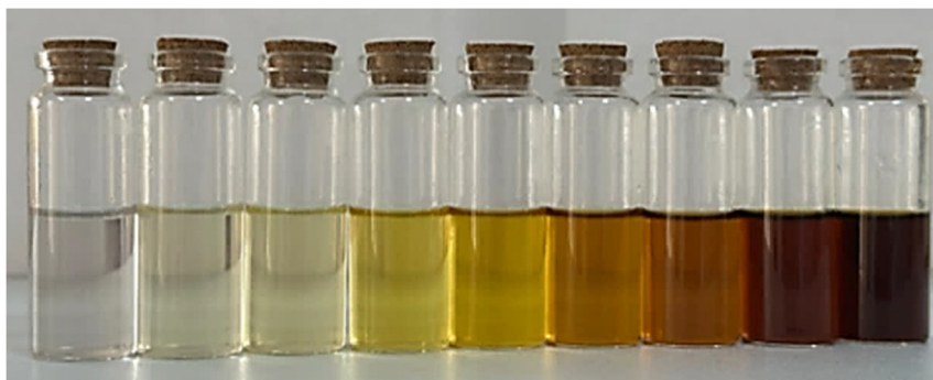
Figure 1. Color change of the Cht- \text{Ag}^0 suspension as a function of reaction time
