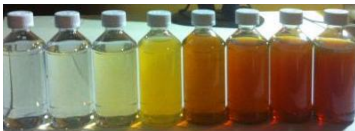
Figure 2. Color of Cht– \text{Ag}^0 suspension depending on the reaction time
