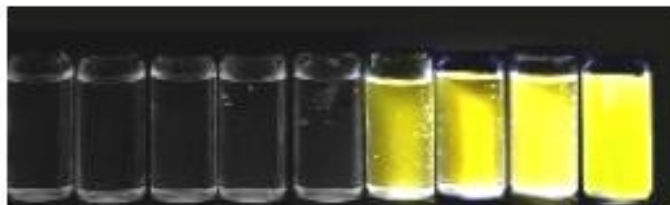
Figure 2.1.3: Images of Zn(II) complex in different volume ratios of water (10-90%) under UV lamp.
