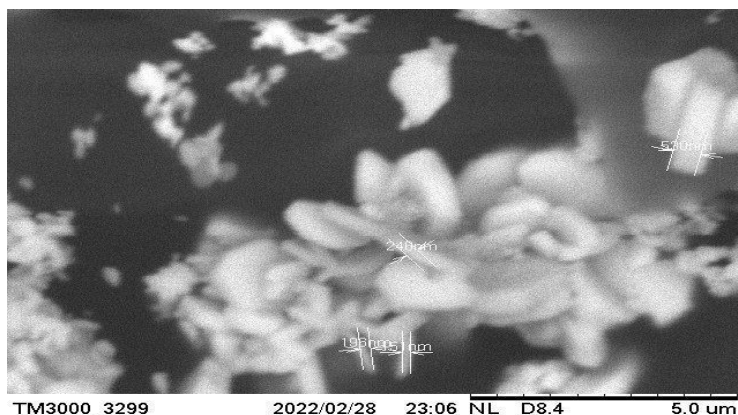
Figure 15. Micrographs of \text{Ag}_3\text{SbS}_4 nanoparticles in a mixture of DMF+TEA.
