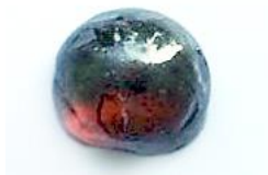
Figure 2. Photo of glass containing (\text{Ga}_2\text{S}_3)_{0.70}(\text{La}_2\text{S}_3)_{0.25}(\text{Nd}_2\text{S}_3)_{0.05} from the \text{La}_2\text{S}_3 - \text{Ga}_2\text{S}_3 - \text{Nd}_2\text{S}_3 quasi-ternary system
