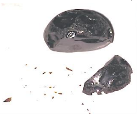
Figure 16. Photo description of the (\text{Ga}_2\text{S}_3)_{0.65}(\text{Nd}_2\text{S}_3)_{0.20}(\text{EuS})_{0.15} glass in the \text{Nd}_2\text{S}_3\text{-Ga}_2\text{S}_3\text{-EuS} quasi-ternary system
