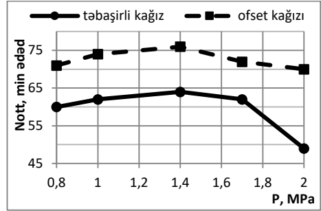
Fig. 19. The graph of the dependence of the circulation resistance - N_{ott} of the impression - process pressure - P
