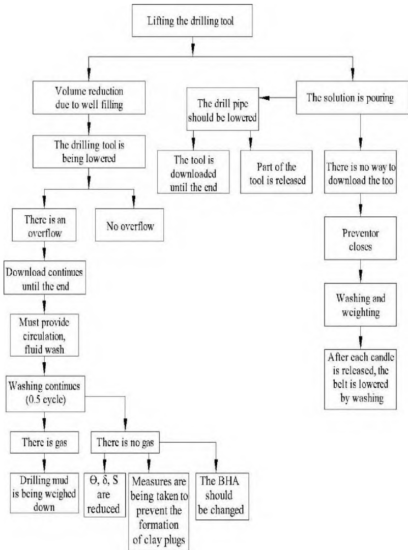
Scheme 6. Block diagram of the algorithm for carrying out measures to eliminate open oil and gas fountains during tool lifting using experimental and mining materials
