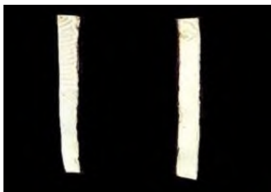
Picture 13. Photograph of 180-day-old nanotalc-based (left) and nanochalk-based (right) enamel surface samples
