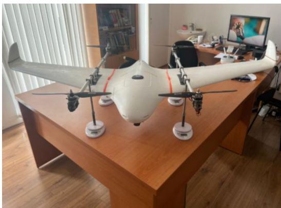
Figure 10. A laboratory-prepared workbench for determining the center of gravity of a VTOL UAV
