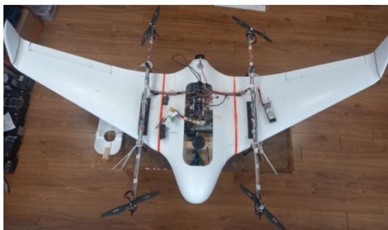
Figure 11. VTOL-type UAV with onboard control and measurement system installed
