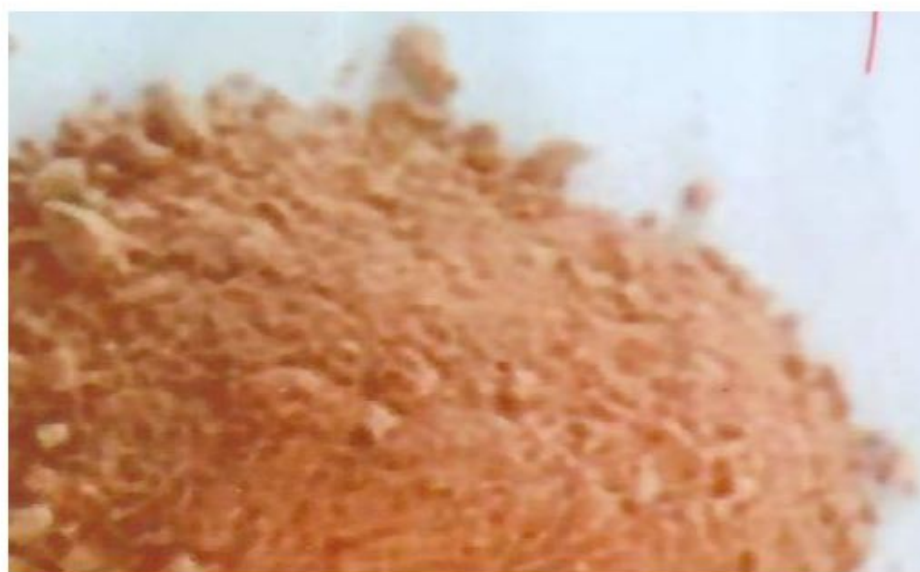
Fig. 1. Mixture of BAF-1 and BAF-2 nanostructured polycrystalline powders
