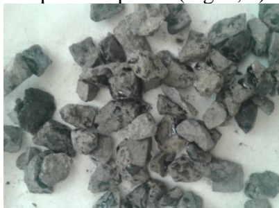
Fig. 3. Test result of road bitumen according to GOST 11508 adhesion 3 points.
