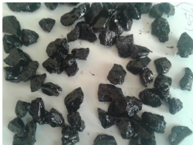
Fig. 4. Test result with the addition of 0.4% of the synthesized additive to road bitumen adhesion 1 point.
