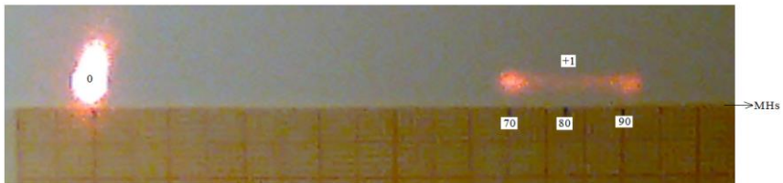
Figure 13. Dynamic positioning of zero and one orders light on the screen
