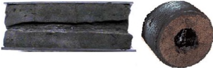
Figure 12. Out-of-state receipt zone created by the RAPS formed in oil pipelines
