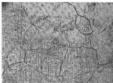
Figure 4. Microstructure of the top layer of 10Г2С1 steel ( \times 800 ) before (a) and after (b) diamond smoothing
