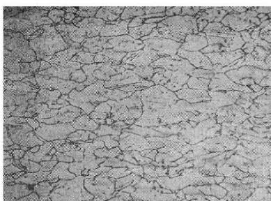
Figure 5. Microstructure of the top layer of ВСТ3сп steel ( \times 800 ) before (a) and after (b) diamond smoothing
