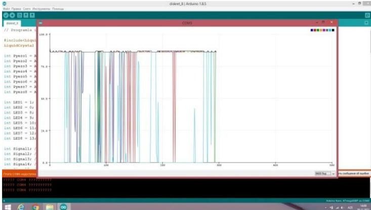
**Figure 5. Computer graph of the voltage at the output of a piezoelectric transducer during vibration**
