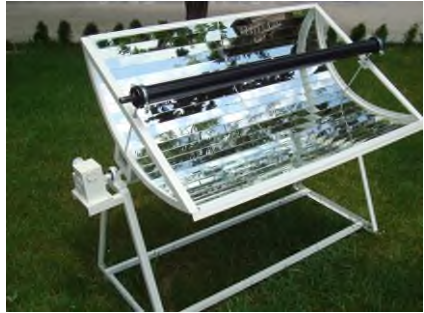
Figure 8. The main view of a solar power plant with parabolic cylindrical concentrator.
