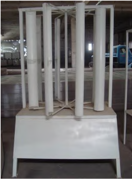
Figure 11. The main view of the multi-blade vertical wind turbine
