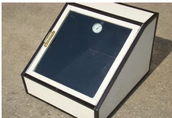
Fig 22. The main view of the solar desalination plant
