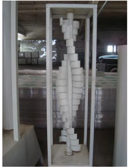
Figure 12. The main view of the multi-blade vertical wind turbine
