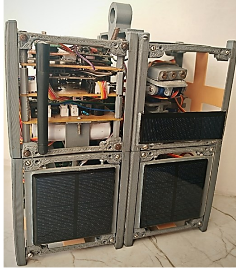
Figure 17. A completed real-world view of the 4U cubesat preliminary engineering model structure
