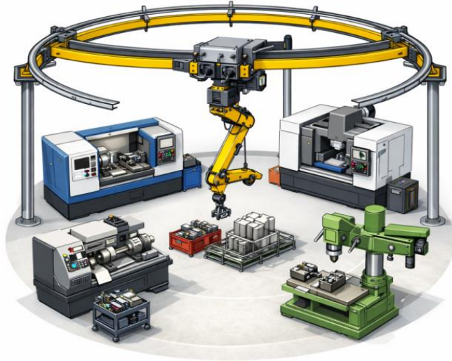
Fig. 4. 3D structure of a module serving several machines of an industrial robot in the field of agile manufacturing
