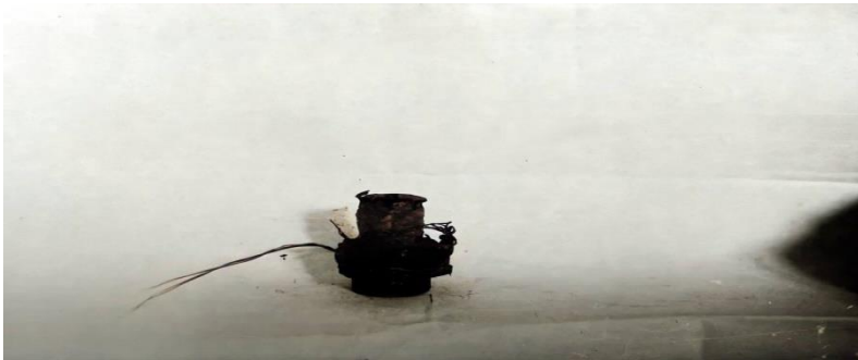
Figure 14. Equipping the milling model with thermocouples
