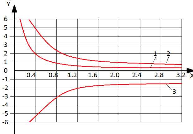
Graph 12. Change of y = \sigma_{rr} - \sigma_{\theta\theta} variation of the voltage difference depending on the “x” parameter ( at different values of \frac{x_1}{x_0} ratio) (Curve 1 \frac{x_1}{x_0}= 0.2 ; Curve 2 \frac{x_1}{x_0}= 0.5 ; Curve 3 \frac{x_1}{x_0}= 1 )
