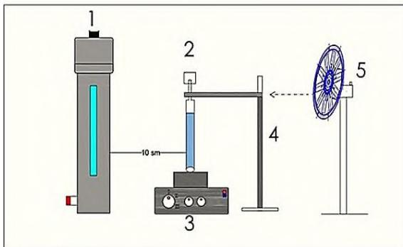
**Figure 1. Schematic of the irradiation process through a UV lamp:
