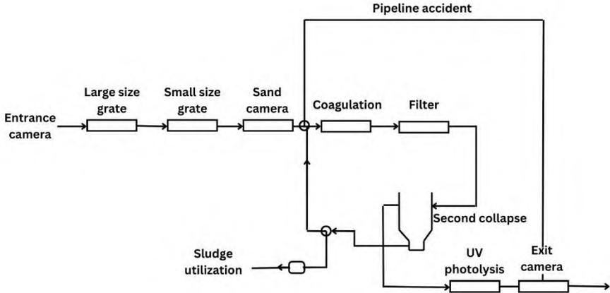
**Figure 3. Production process flow chart**
