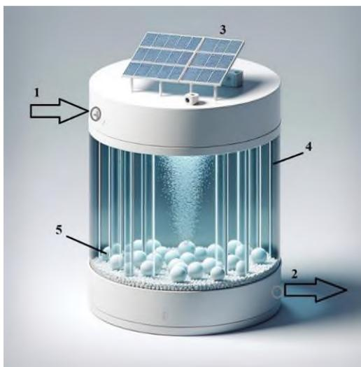
**Figure 4. The principle scheme of the cleaning device. 1-Inlet water, 2- Outlet water, 3-Solar panel, 4-UV lamp, 5-N-TiO<sub>2</sub> catalyst**
