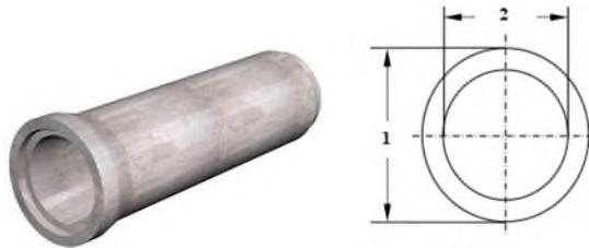
**Figure 2. Image and dimensions of a reinforced concrete pipe; 1-D1800 mm, 2-D1300 mm**
