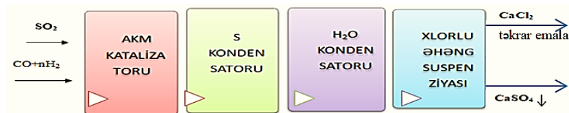
Figure 3 Schematic technological scheme of absorption of the remaining gas mixture (H 2 S, SO 2 , N 2 , CO 2 ) with chlorinated lime after reduction of SO 2 with conversion gas
