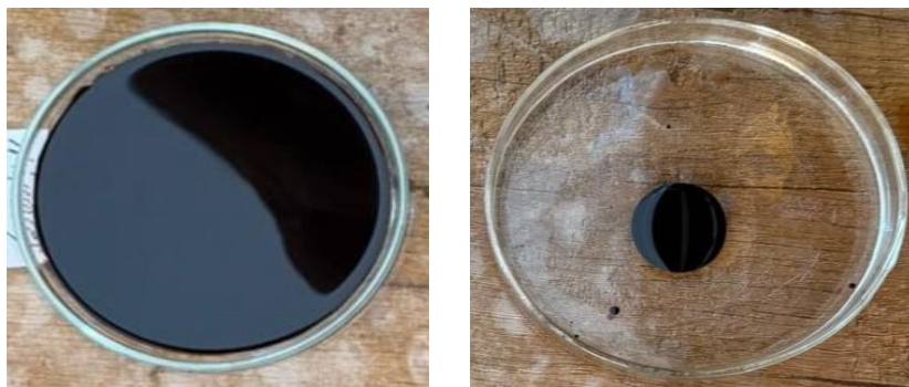
Figure 3. Oil-collecting capacity of the IPA + nitration product of diesel distillate + Fe salt of NPA composition for Salyan oil from the water surface
