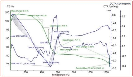
Figure 6. TG/DTA/DDTA spectra of a sample belonging to Upper Maykop.
